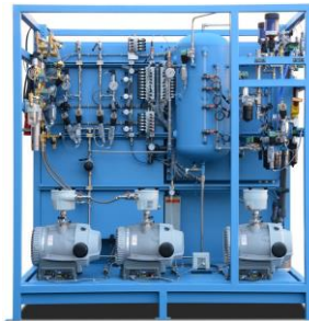
Rear View showing dry scroll vacuum pumps, S/S piping, dehydration and storage tanks
