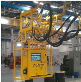
DataFill MultiFill System for Transmission, Diesel Fuel, Engine Oil, Coolant and Axle
