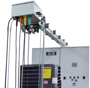
Test Connector Panel Mounted on Rotating Boom
