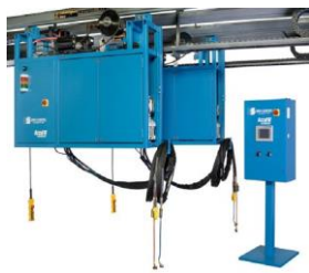
Overhead rail mounted AccuFill A/C Fill System with VFD motors
